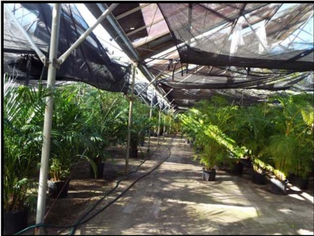
This building is 75 x 100 feet, concrete floors with drainage areas and it is steel framework that is easy to adapt to and has only had hurricane damage to the shade cloth and poly coverings.
